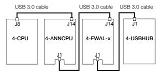
The 4-USBHUB's J1 connector may be connected directly to a 4-CPU, 4-ANNCPU, 4-NET-AD, 4-CPU-GRPH, or 4-FWAL and must always be the last device on the data bus.
